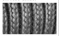
This innovative compression packing for control valves is proven to reduce VOC emissions, it has a long term, high integrity sealing capability with very low stem friction for control accuracy. Made of high purity graphite, reinforced with a non-metallic structure for additional strength and resistance.
