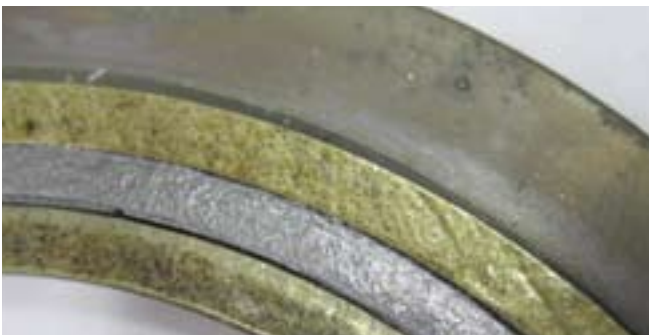
Lamons Kammpro HTG after exposure to 1500°F - The flexible graphite maintains all its physical and mechanical properties after exposure.
