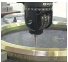
Accuracy and precision throughout the production process is rigorously checked.
