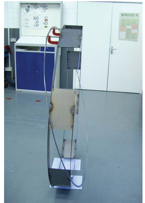
The Novus test rig designed to replicate the dimensions of the tube sheet and the restriction caused by the tubes.
